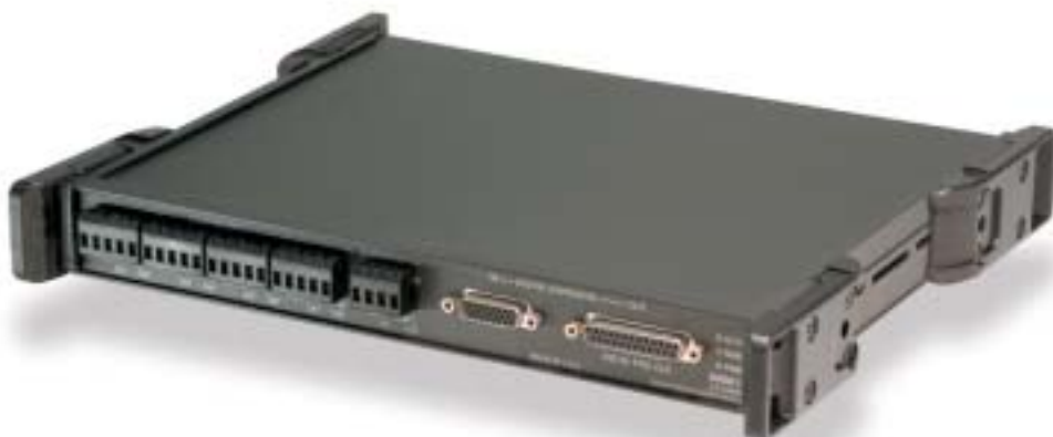
The WBK17 provides eight channels of 32-bit general-purpose counters, and is also capable of multi-axis quadrature encoder monitoring
